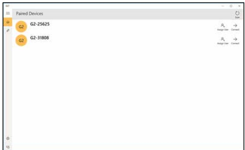
5. Locate the instrument you wish to connect to, and select the connect option. A loading animation should appear to the left.
