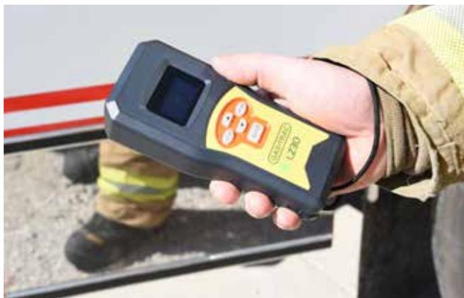
TDLAS uses a laser that is tuned specifically to detect methane, the major component of natural gas. The laser beam emits a specific wavelength which is absorbed by methane. When the laser's path crosses methane molecules, some laser energy is absorbed. The detector analyzes the difference between the laser light energy that was sent to what was reflected to the sensor. The result is displayed in ppm-m (parts per million meter).
