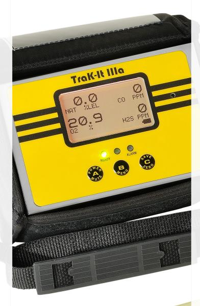
7. The combustible gas scale will automatically range from %LEL to %Volume if so equipped with the 100%v/v (TC) sensor.
