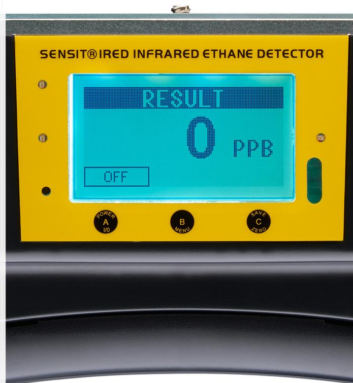
9. You are now ready to use the instrument. "For Best Results: Using a gas detection device capable of sensing low level natural gas concentrations, confirm a gas measurement in a range of 50 - 2000ppm prior to use of the IRed"
