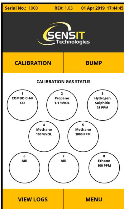
**NOTE:** For calibration and bump test records to be downloaded from the SMART-CAL 360 with either SCAL-D 360 or SCAL-N 360, the station must be powered on and on the "Home Screen", as pictured.
