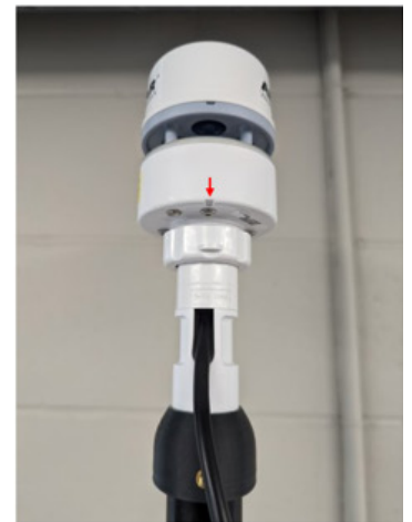
Install MET ( Notch must point North)
