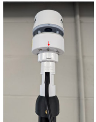
Install MET (Notch must point North)
