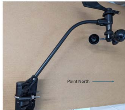
Install MET ( Notch must point North)
