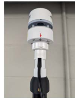
Install MET ( Notch must point North)
