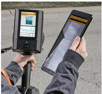
The GAS•TRAC® LZ-50 is an innovative handheld methane gas detector that provides instantaneous readings from a distance to the target of up to 164'. Its revolutionary laser photonics combined with breakthrough technology, TARGETGPS, (COMING SOON) makes it the clear choice in remote laser methane detection.
