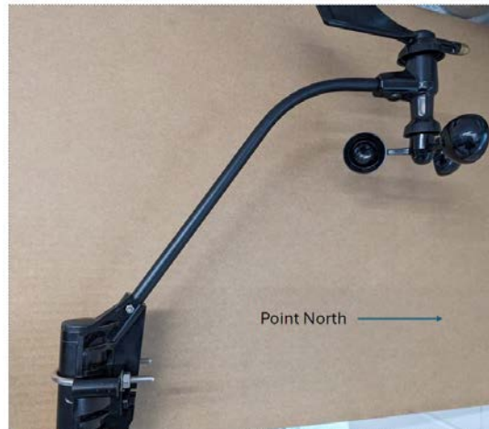
Install MET ( Notch must point North)
