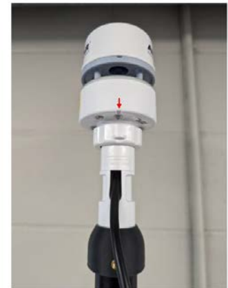
Install MET ( Notch must point North)
