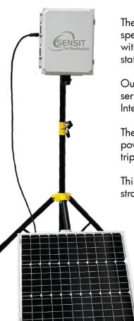
The **GAS** • **TRAC**® **FMD** is an active sampling system equipped with a tunable diode laser spectroscopy (TDLAS) cell capable of detecting methane as low as 200 PPB. When equipped with an anemometer, the **FMD** is capable of localizing leaks, as well as providing state-of-the-art data to aid in quantification.
