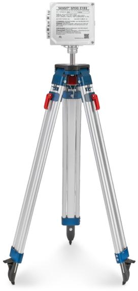
The **SENSIT® SPOD C1D2** is an advanced, low-cost sensor system that can be powered by solar panels. It can detect volatile organic compound (VOC) emission or natural gas (Methane) plumes by combining wind and air pollutant concentration measurements, thereby making it easier to locate the source of emissions.
