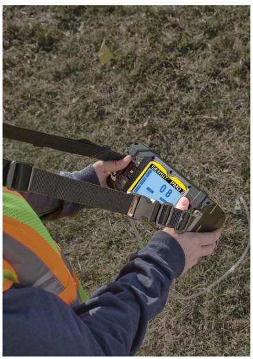
The **SENSIT® PMD2** is a compact, lightweight, advanced methane detector used to pinpoint and grade leaks. With TDLAS detection technology, the **SENSIT® PMD2** is methane selective and perfect for walking or vehicle applications.
