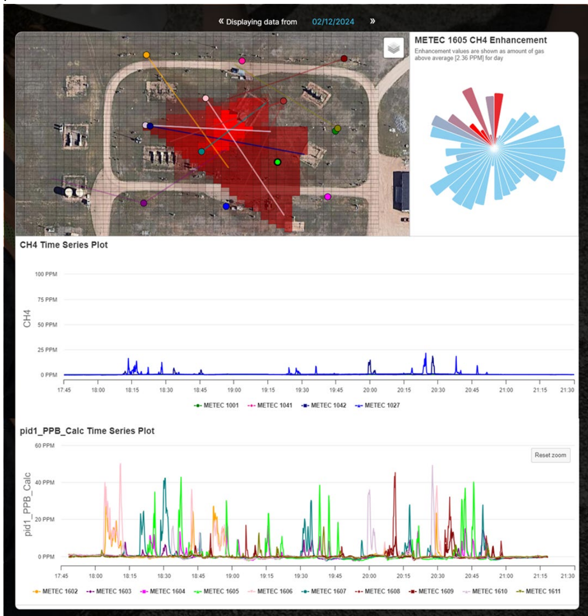
Fig. 6 – Sample image of SENSIT's leak localization algorithm. Within the map, the areas of greatest red indicate the area with the highest probability of a leak. In this case, the tank asset at the center of the site was indicated as leaking – this was subsequently confirmed after the results were released.
