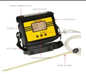
TRAK-IT® IIIa instruments are constructed of durable stainless steel to withstand the rigors of field use.
