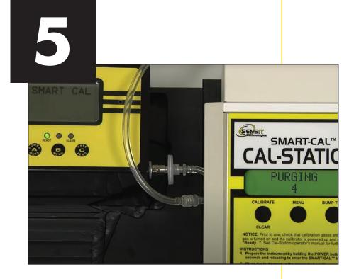
Screen will display PURGE countdown. After PURGE is complete, instrument will AUTOZERO and calibration process will begin.
