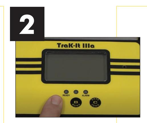
Attach Instrument Hose & Press & Hold A to Power on the Trak-It IIIa
