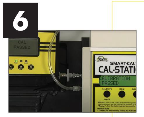
Continue Calibration until SMART CAL displays "CALIBRATION PASSED". If there is a problem or failure, repeat procedure. If the calibration failure persists, contact SENSIT's Repair Department at 219-465-2700
