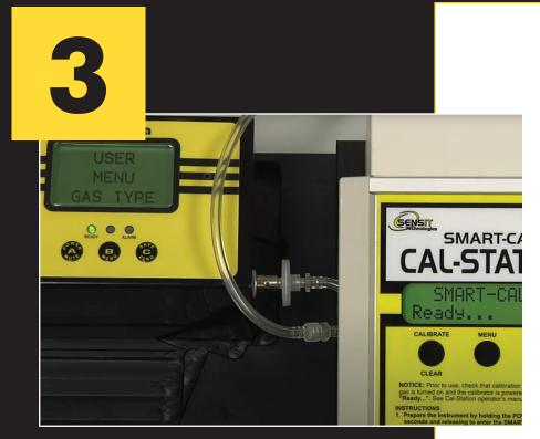
To Change GAS TYPE, Press & Hold B, then Press & Release C to scroll to GAS TYPE. To select gas, Press & Release B for NAT or C for PRO. Press & Release A to return to working display.
