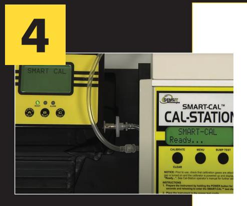
Allow instrument to warm up for 5 minutes. To enter into SMART-CAL, Press & Hold A for 2 seconds. On Cal Station, Press & Release Calibration Button.
