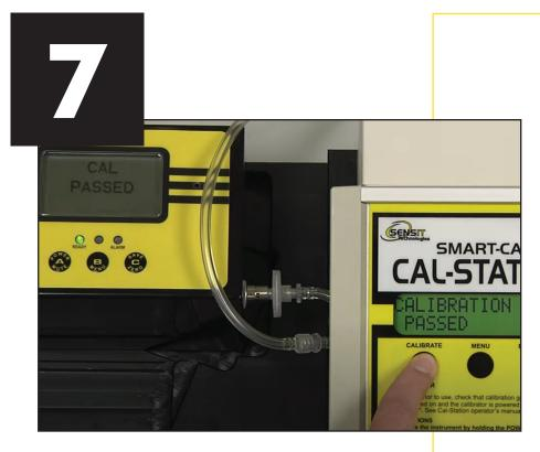
Once PASSED, Press & Release the Clear Button on the Cal-Station. Trak-It Illa will return to working display, Press & Release A. Disconnect hose and allow instrument to purge before turning off.
