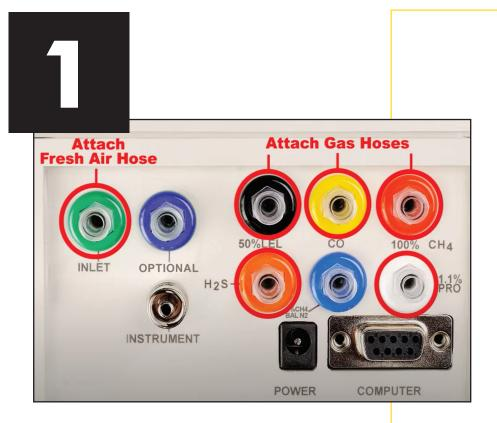
Attach Fresh Air Hose and Gas Hoses to Smart-Cal Station
