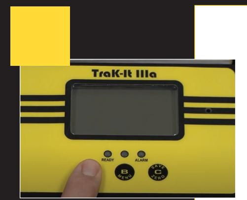
Attach Instrument Hose & Press & Hold (A) to Power on the Trak-It IIIa
