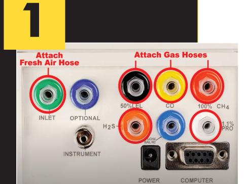
Attach Fresh Air Hose and Gas Hoses to Smart-Cal Station
