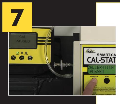
Once PASSED, Press & Release the Clear Button on the Cal-Station. Trak-It Illa will return to working display, Press & Release A. Disconnect hose and allow instrument to purge before turning off.
