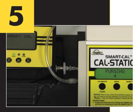
Screen will display PURGE countdown. After PURGE is complete, instrument will AUTOZERO and calibration process will begin.
