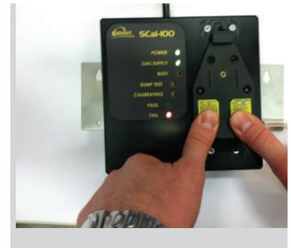
The BUMP and GAS LED's will illuminate indicating gas is being applied for the bump test.
