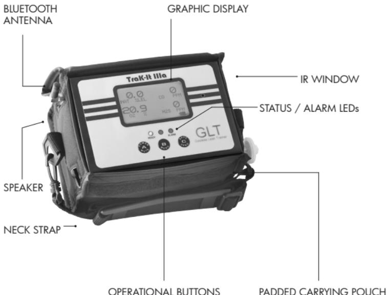
**TRAK-IT® IIIa GLT** instruments are constructed of durable stainless steel to withstand the rigors of field use.
