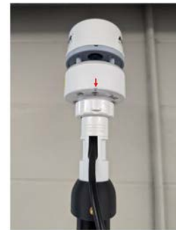
Install MET (Notch must point North)
