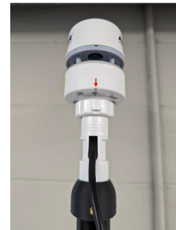
Install MET (Notch must point North)
