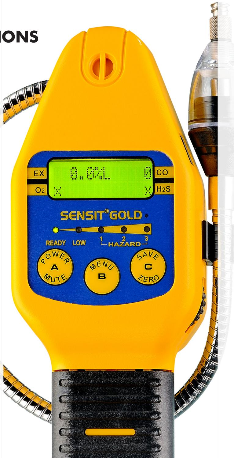
7. Extend the goose neck (the LEL sensor and filter cap is at the tip).
